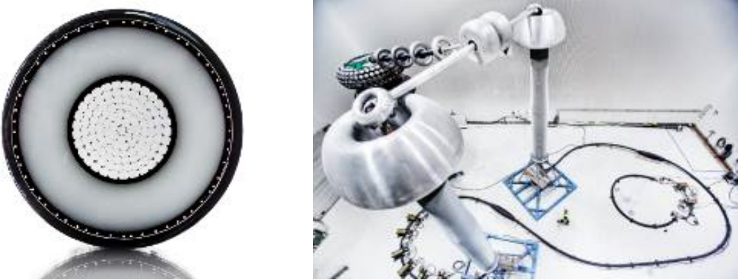
Figure 2 .a) Cross-section of a 525 kV extruded XLPE DC Cable. b) Type testing of the same cable in a cable system with joints and terminations [Copyright ABB]
