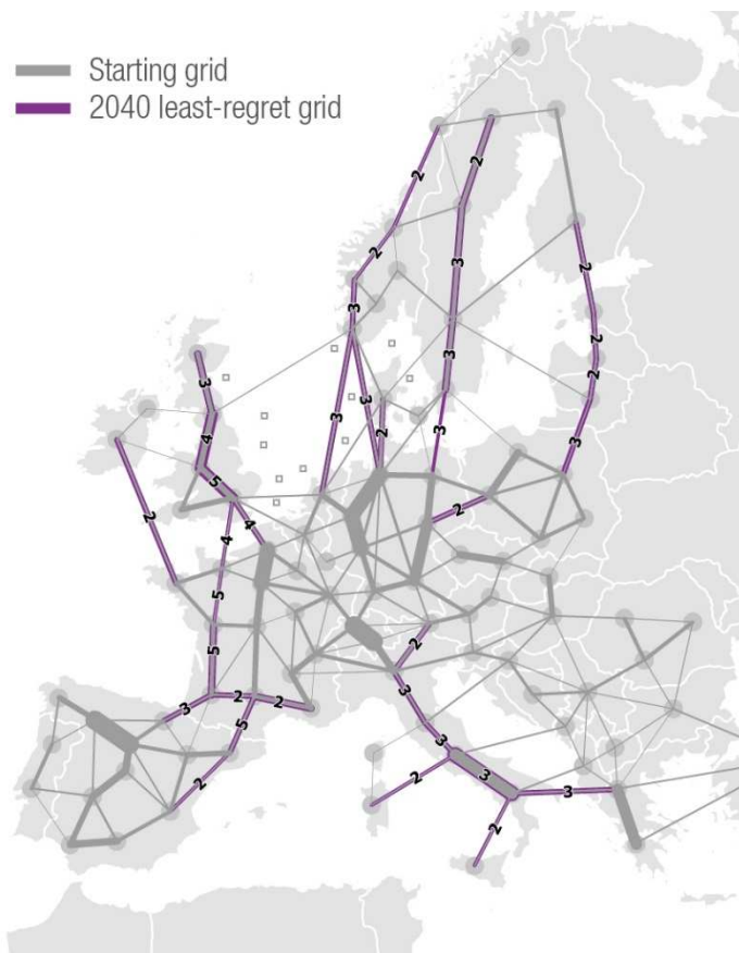
Figure 6: grid architecture for 2040, robust to the 5 scenarios (grey: starting grid, purple: reinforcements)
